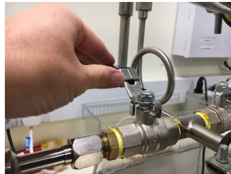
Lifting metal piece to unlock LH valve
