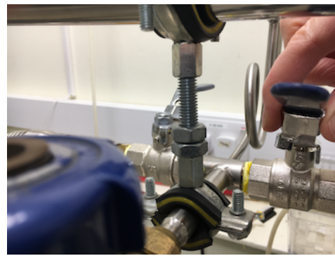
Lifting metal piece to unlock RH valve
