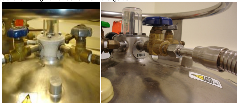
Figure 9: Blue valve for feeding LN2 to small dewar.
