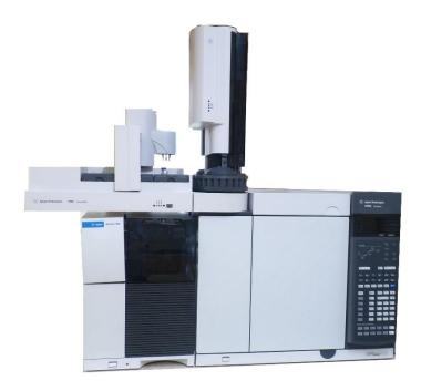
There are two Agilent quadrupole GCMS's, the 6890N GC with 5973 MS with Mass Selective detections and the 7890A GC with 5975C MS with a triple axis detector. These are perfect for the selected ion monitoring of stable-isotope tracer enrichment in any cell, blood or tissue fraction and currently used for labelled fatty acid and glucose analysis.
