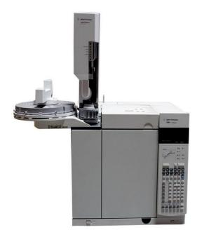
There are two Agilent Gas Chromatography machines, a 6890N and 7890B. Equipped with flame ionisation detection, it allows the fatty acid composition of specific fractions from cells, blood and tissues to be determined.
