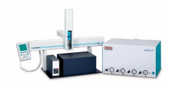
The Thermo Scientific™ GasBench II universal on-line gas preparation and introduction system facilitates high-precision on-line isotope and molecular ratio determination of headspace samples, and is used for allows for water equilibration. It is used for measurement of deuterium enrichment in plasma, urine, saliva and cell media.
