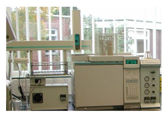
The Finnigan GC-C/TC III interface is a state-of-the-art GC interface and is used for the analysis of <sup>13</sup>C/<sup>12</sup>C. Organic compounds elute from a GC6890N column and are then converted into simple gases when traversing a capillary micro-reactor. Accordingly, all compound specific isotope ratios can be analysed in the IRMS. This is utilised for analysing the enrichment in breath, blood and tissue samples after consumption of a 13C stable-isotope tracer.
